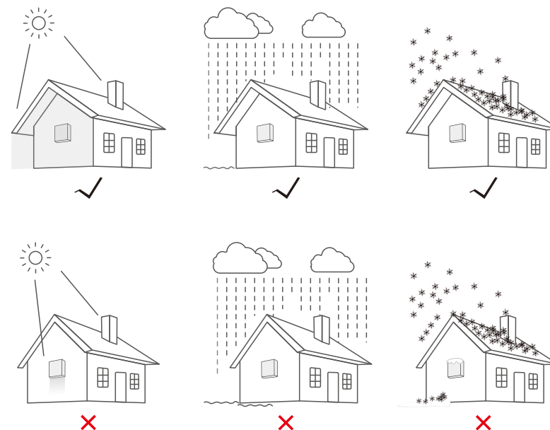
▲ Figure 4.1 Recommended Installation locations
